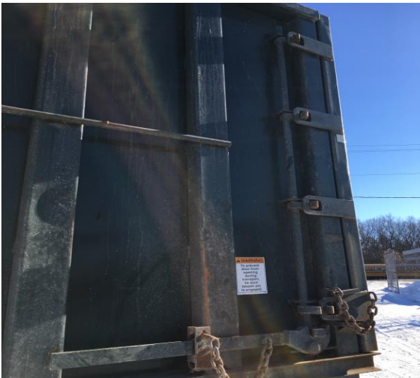
Cam lock system, with vertical handle
